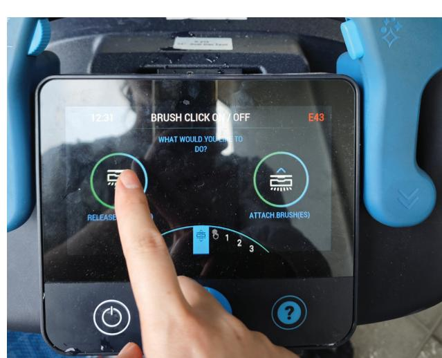
15. Press the RELEASE BRUSH button and wait for the brush/pad holder to fall on the floor. Remove to clean or change brush.
