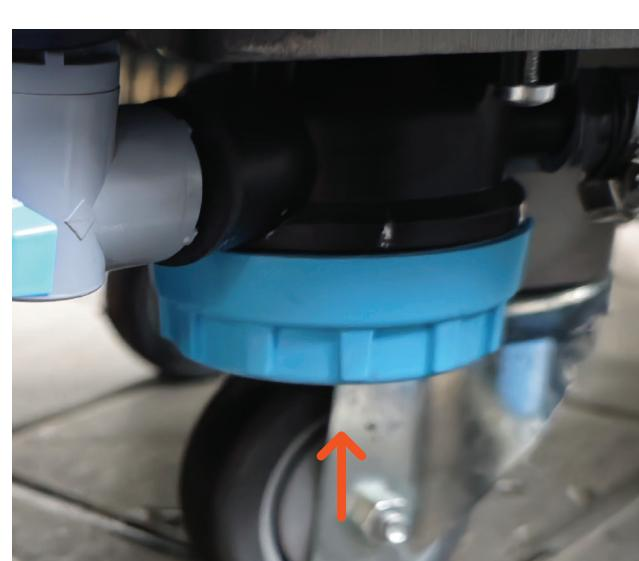
3. Check if the solution filter is cleaned and the solution valve is open.
