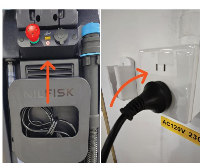
19. Charge the batteries: Take the cable out of the cable box, and connect the battery charger cable to the electrical socket.
