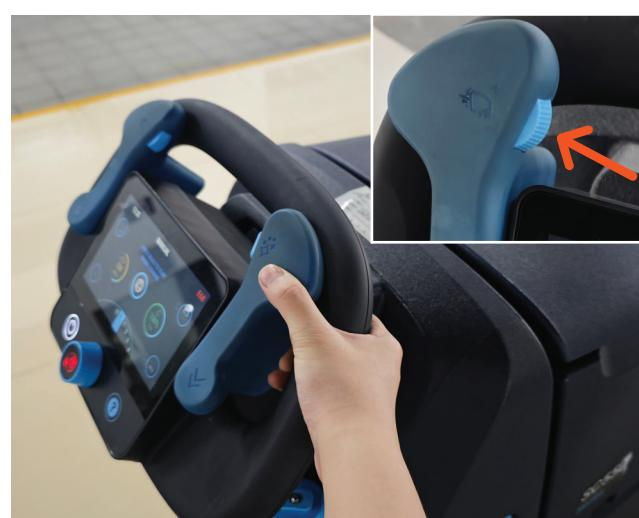
8. Push forward the drive paddle to start cleaning. Adjust maximum speed by the speed control knob.
