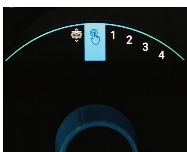
11. There are 6 modules for knob selection; the first one is set up and down the brush; the second is manual control; and the last four are preset cleaning models.
