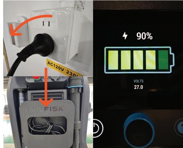
1. Disconnect the battery charger cable from the electrical socket. Then place the cable into the cable box.
