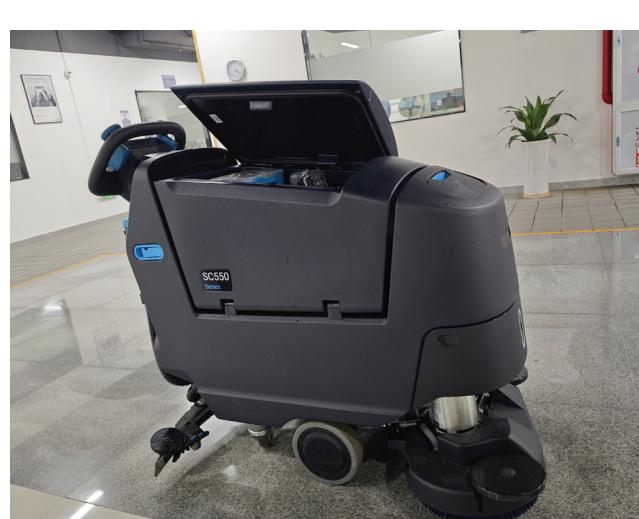
20. Park the machine with the recovery tank cover open.
