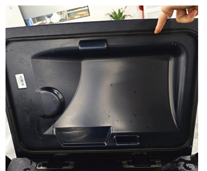
4. Check the lid gasket is in good and working condition and sealing when lid is closed.
