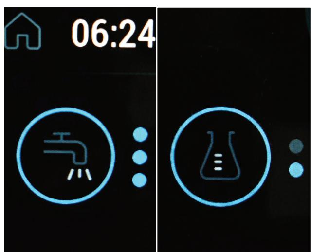
9. To change the solution flow level push the solution button and change flow level according to the cleaning performance and application. (Only setting in manual mode).
