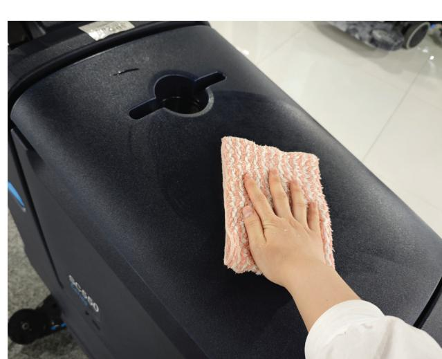
18. Clean the machine using a damp cloth and where needed use a neutral cleaning product.
