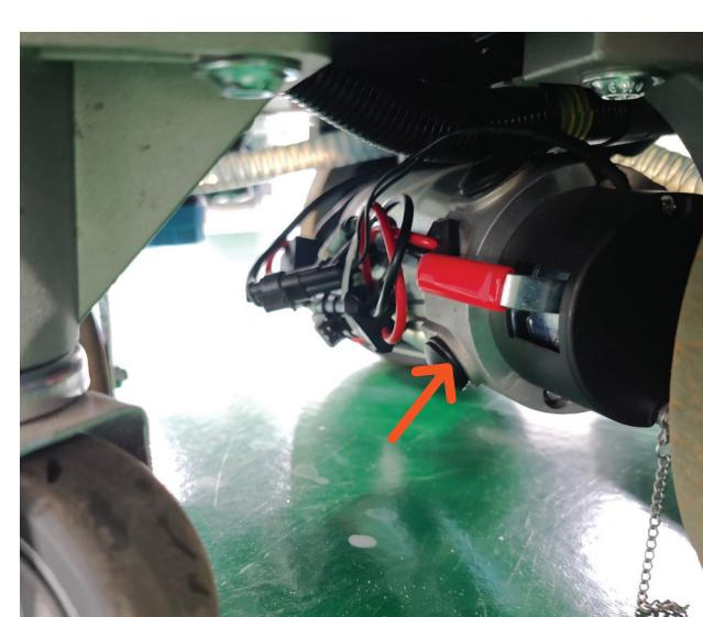
2. Check if the brake on the drive motor is lifted.
