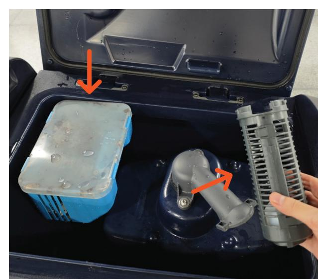
2. Open the recovery tank and check the debris tray and float are clean and working.
