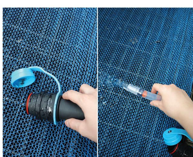
12. Empty the recovery tank with the hose. Then empty the solution tank with the transparent hose.
