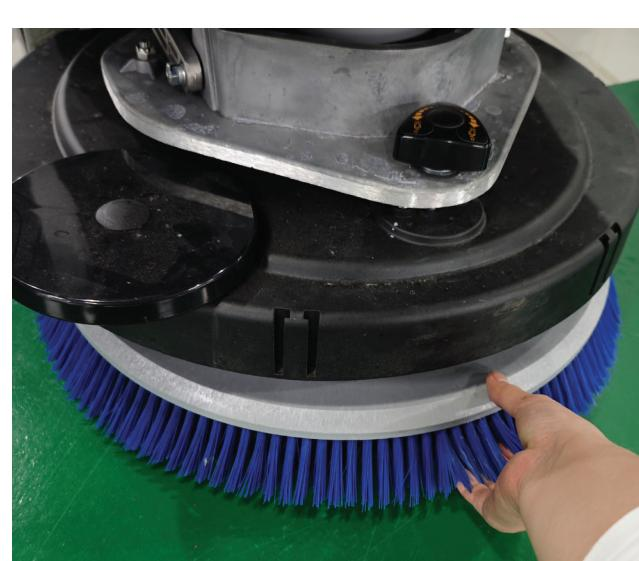
3. Check if the brush are correctly installed and not worn out or if there are external materials avoiding brush rotating.
