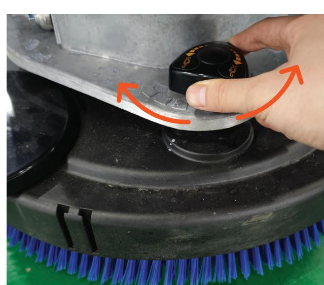
1. To adjust machine direction turn front knob until machine is working straight.
