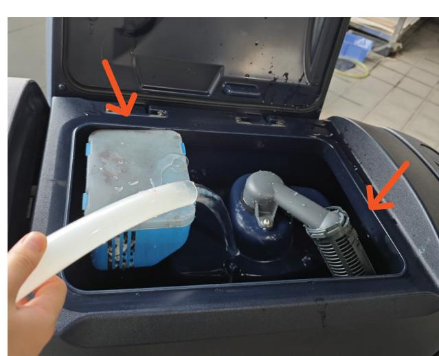
13. Empty the debris tray and clean/wash the recovery tank inside.
