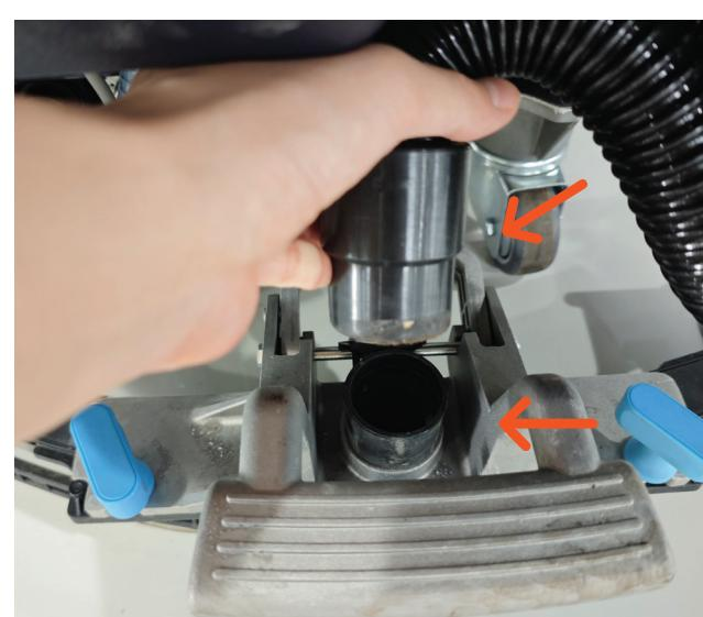
1. Check if the suction hose is correctly installed and cleaned.
